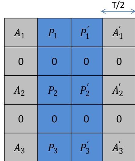
Fig. 4. Pair of Pilots based Preamble structure
